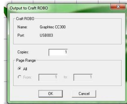
The first prompt will ask you to confirm how many copies, also check that is connected to the right device (Graphtec CC3xx [xx being the model number]). Now click OK button to proceed.
